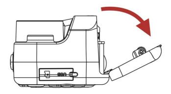
2. Insert the paper roll into the paper tray as shown.
