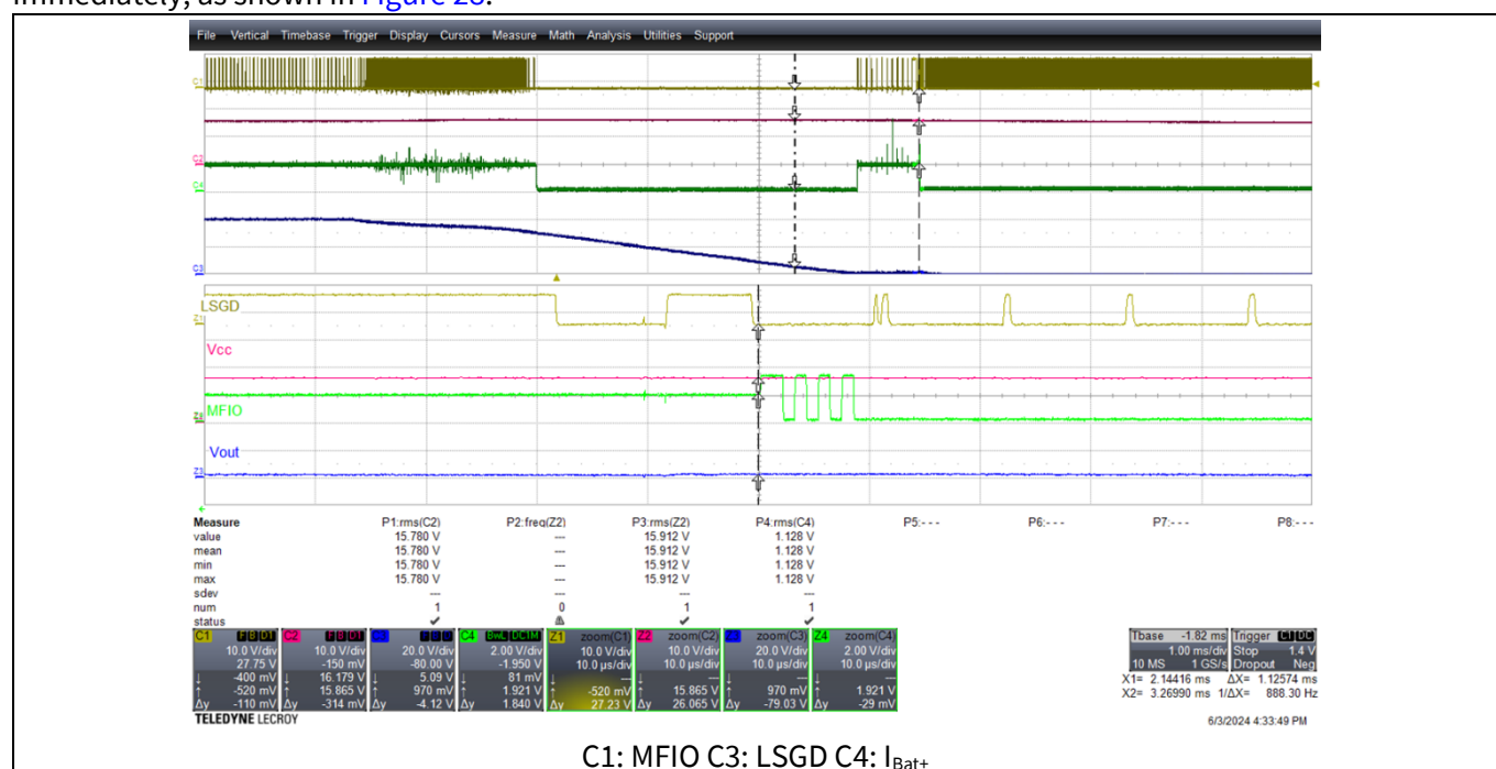
Figure 28 Vout_UVP triggering at short circuit event at the output
