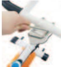
3. Fix the handlebar to its support with the Allen screws and washers.
