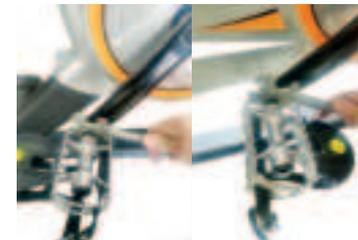
2. The pedals are marked "L" (left) or "R" (right). Insert the fixing screw of the right pedal into the crank on the right side of the product and fix it with the spanner. Then, screw the nut into the fixing screw on the other side of the crank. Proceed the same way to fix the left pedal to the crank on the left side of the product.
