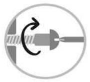
Turn clockwise to tighten and only tighten when step is completed or when instructed to do so.
