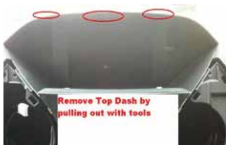
Remove top panel (pulling out with tools)
