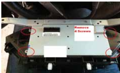
Remove 4 screws Take out LCD Panel
