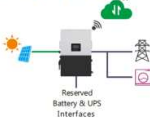
C. On-grid solar system without battery (Powers loads even without battery)
