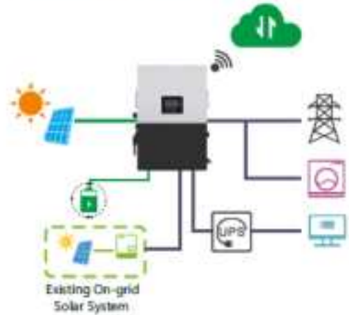
B. AC Coupling with existing solar system
