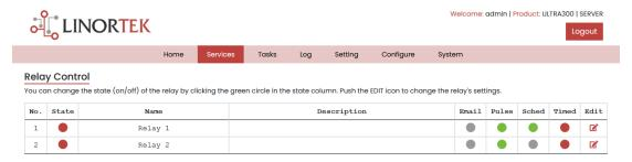
The **State** LED show whether the relay is on or off indicated by GREEN and RED respectively. This icon is clickable to manually control the corresponding relay. Each relay can have a Name as well as identifiers for the Normally Open, Common and Normally Closed connections.
