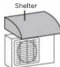
Build a shelter to protect the unit
