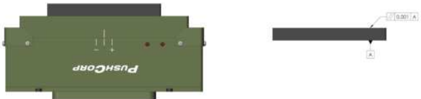
Figure 2: Carriage Mount Bracket - Parallelism
