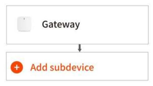
3.Press the reset button for 5 seconds, till the screen blink, then click the confirm button which shows and "LED already blink" follow the in-app instructions to connect the sensor to your gateway.
