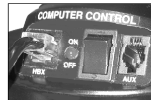
Fig. 12: Connect Autostar to the HBX port.
