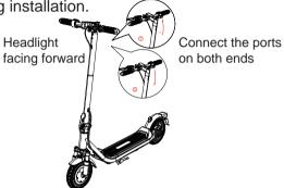
4. Conduct turn on and off detection after installation
