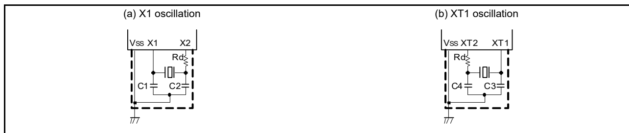
Figure 6 - 23 Examples of External Circuits
