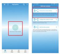
3. After switching to the WiFi connection page, select the corresponding WiFi hotspot and connect. After the connection is successful, return to the APP, and the device is added successfully. (If the APP does not automatically add a device, click Search to add the searched device)
