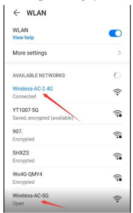
3. After connected to Wireless-AC-2. 4G or Wireless-AC-5G, phone will open the admin page automatically, type user name: admin, password: admin. (If not open, or if using computer, please manually open a browser and type the IP address 192. 168. 100. 99 in address bar to enter into admin page. User name and password are both admin, all lower case)
