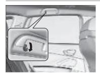
There are coat hooks on the rear grab handle of both sides. Pull it down to use it.
