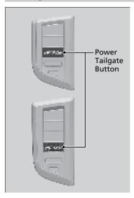
Press the power tailgate button for more than one second to operate when the power mode is in VEHICLE OFF.
