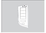
Red LED: Blinks when the keyless remote is out of the keyless system range. The engine will not stop.
