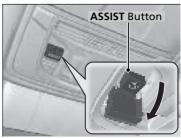
If you need to talk to the AcuraLink operator in a situation where no airbag has deployed, you can manually connect to them by pressing the **ASSIST** button with the power mode in ACCESSORY or ON.
