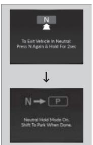
If the **ENGINE START/STOP** button is pressed after car wash mode has been activated, the power mode will change to ACCESSORY and a message will be displayed on the multi-information display.
