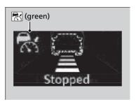
If no vehicle is ahead of you before you resume driving, depressing the accelerator pedal will resume operation of ACC with Low Speed Follow within the prior set speed.
