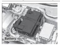
The condition of the battery is monitored by a sensor located on the negative terminal of the battery. If there is a problem with this sensor, the multi-information display will display a warning message. If this happens, have your vehicle inspected by a dealer.
