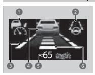
You can see the current state of ACC with Low Speed Follow, and Lane Keeping Assist System (LKAS).
