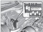
Remove the cover on the  $\oplus$  terminal (as shown).
