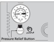
**11.** Press the pressure relief button until the gauge returns 0 psi (0 kPa).
