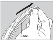
**2.** Slide the wiper blade out from the end with the indent.
