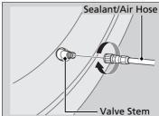
**7.** Attach the sealant/air hose onto the tire valve stem. Screw it until it is tight.
