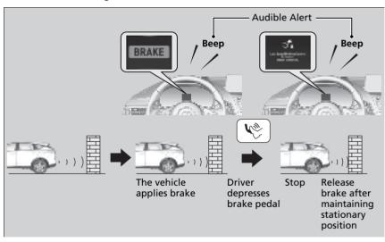
If only the rear sensors are turned off using the parking sensor system, the assistive braking will not work when reversing.
