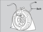
**4.** Bore through the bag, and pass the holding belt through the hole of the bag and the wheel of the flat tire as shown.
