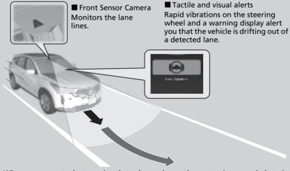
When you operate the turn signals to change lanes, the system is suspended, and resumes after the signals are off.
