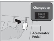
Depress the accelerator pedal while the transmission is in a position other than  $\boxed{\mathbf{P}}$  or  $\boxed{\mathbf{N}}$ . The system is canceled and the vehicle starts to move.
