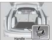
**1.** Push the rear edge of the handle on the floor lid and open the lid.
