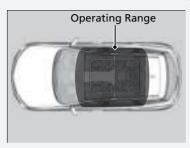
You can start the engine when the keyless remote is inside the vehicle
