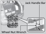
**5.** Put the wheel nut wrench with the jack handle bar on the hoist shaft.
