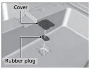
**4.** Remove the cover and the rubber plug on the cargo area lining to access the shaft for the compact spare tire hoist.
