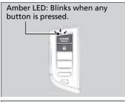
Press the <u>a</u> button, then press and hold the <del>m</del> button.
