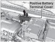
**1.** Open the fuse box cover on your vehicle's 12-volt battery positive  $\oplus$  terminal.
