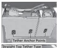
A tether anchor point is provided behind each rear seating position.
