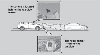
The system starts monitoring the roadway ahead when your vehicle speed is about 3 mph (5 km/h) or above and will search for a vehicle in front of you.
