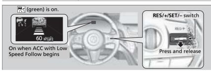
When driving at about 25 mph (40 km/h) or above: Take your foot off the pedal and press down the RES/+/SET/– switch when you reach the desired speed. The moment you release the switch, the set speed is fixed, and ACC with Low Speed Follow begins.
