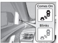
Blind spot information system alert indicator: Located near the pillar on both sides.
