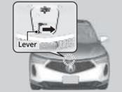
**3.** Push the hood latch lever (located under the front edge of the hood to the center) to the side and raise the hood. Once you have raised the hood slightly, you can release the lever.
