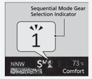
The transmission is in  $\boxed{\textbf{S}}$  and **Sport** mode, to prioritize the engine performance enhancement, the transmission may not allow for shifting up while the engine speed is low.
