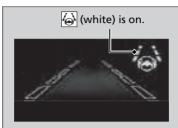
When the LKAS is suspended, the lane lines on the multiinformation display change to lane outlines, and the beeper sounds (if activated).
