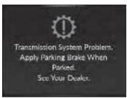
■ Reasons for the indicator to blink The transmission is malfunctioning.
