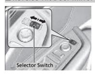
If activated, either side door mirror automatically tilts downward when you put the transmission into  $\mathbb{R}$ ; this improves close-in visibility on the selected side of the vehicle when backing up. The mirror automatically returns to its original position when you take the transmission out of  $\mathbb{R}$ .
