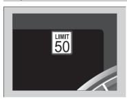
Shows the current speed limit based on either information compiled through the navigation system\* or speed limit signs captured by the front sensor camera.
