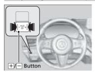
When the power mode is in ON, you can use the  $\boxed{+}/\boxed{-}$  button to adjust head-up display brightness.
