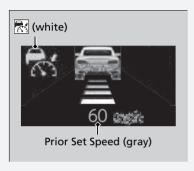
The set speed cannot be set or resumed when ACC with Low Speed Follow has been turned off using the button. Press the button to activate the system, then set the desired speed.
