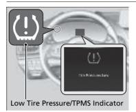
Monitors the tire pressure while you are driving. If your vehicle's tire pressure becomes significantly low, the low tire pressure/TPMS indicator comes on and a message appears on the multi-information display.
