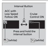
Press and hold the interval button for one second. **Cruise Mode Selected** appears on the multi-information display for two seconds, and then the mode switches to Cruise. The comes on.
