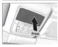
To open the sunglasses holder, press and release the indent. To close, press it again until it latches.
