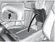
Slide the armrest to the rearmost position. Pull the handle to open the console compartment.
