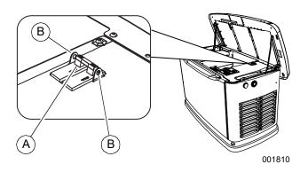
Figure 3-4. Main Line Circuit Breaker (MLCB)
