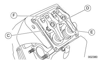
Figure 4-8. Valve Clearance Adjustment (20-24 kW)
