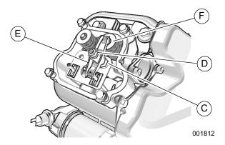
Figure 4-7. Valve Clearance Adjustment (10 kW)
