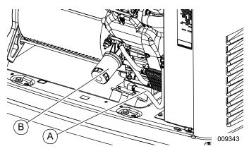
Figure 4-3. Oil Filter and Drain Location (20-24 kW)
