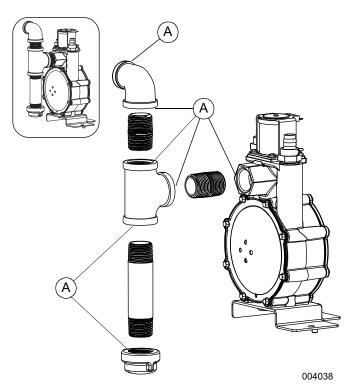
Figure 4-12. Connection Points to Leak Check
