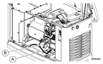
Figure 4-2. Oil Filter and Drain Location (14-18 kW)
