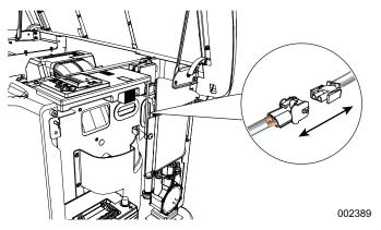
Figure 4-9. Disconnecting Battery Charger Cable
