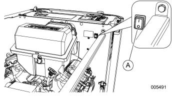
Figure 3-7. Internal Auxiliary Shutdown Switch (14–24kW)
