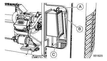
Figure 4-4. Servicing Air Cleaner (10 kW)
