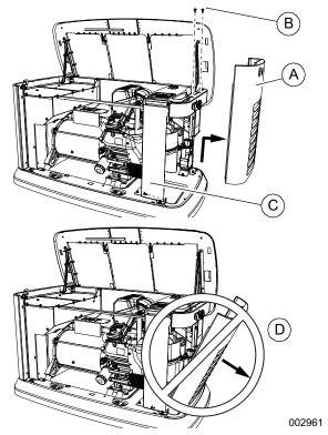
Figure 3-3. Intake Side Panel Removal
