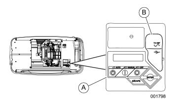
Figure 3-8. Generator Control Panel
