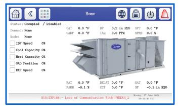
Single-zone cooling and heating demands can be established based on an accessory space temperature (SPT) sensor or 2-stage heat/cool thermostat inputs.
