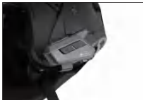
② Slide the mount into the slot of the intercom
