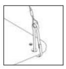
1. Attach the clips on the ends of the hanging wires to each of the hanging holes on the light.
