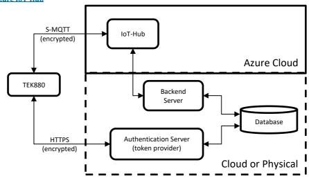
The TEK880 sends payload messages to the backend server using the IoT-Hub service as a broker. Since the IoT-Hub is a highly secure service, it requires devices to authenticate themselves on each connection. The existence of a secondary web service to manage the authentication credentials, here called authentication server, is essential to guarantee a secure and reliable ecosystem.
