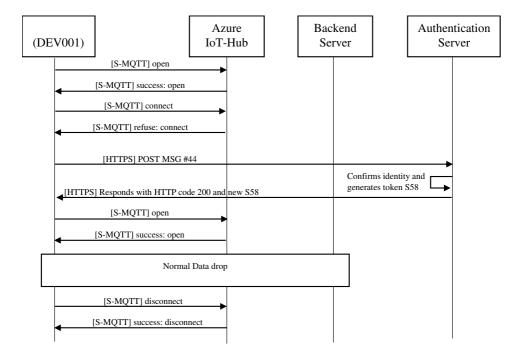
After contacting the authentication server and receiving a new token, if the S-MQTT connection with IoT-Hub is refused again, the device will ignore the transaction and return to a dormant state until the next scheduled contact, to save battery. The same will happen if the HTTPS response code from the authentication server is anything other than 200.
