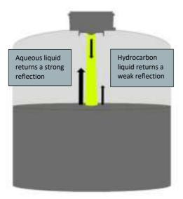
**Note** – The signal strength can vary due to external factors such as condensation or whether the sensor installation is non-invasive or invasive (with the signal passing through the tank wall). As such it is important the sensor is installed as flat as possible.
