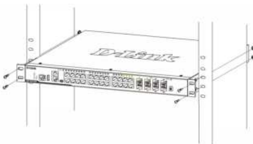
Figure 3 — Installing the Switch in a Rack
