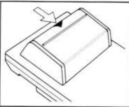
Connect the poles of the battery supplied (Type 6 F 22, 9 V) with the push button contacts in the battery housing.
