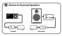
**Note:** If you have Audioengine 5+ powered speakers, you may use the built-in USB power/charge port on the A5+ to power the W3 Receiver. Otherwise, you can use an iPhone charger or purchase an extra Audioengine power adapter.
