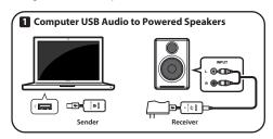
Note: If using Audioengine 5+ (A5+) powered speakers the A5+ USB power port can be used to power the W3 Receiver
