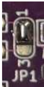
Step 2 Completed Bridge
