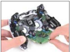
Carefully guide the joysticks through the front case and lift the motherboard out.
