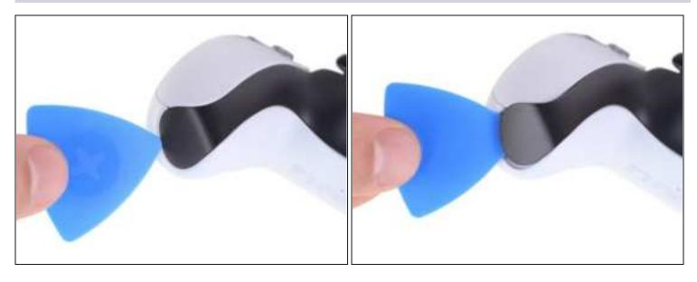
• Insert an opening pick underneath the middle trim at the bottom-left corner of the controller to release the clips securing it to the case.
