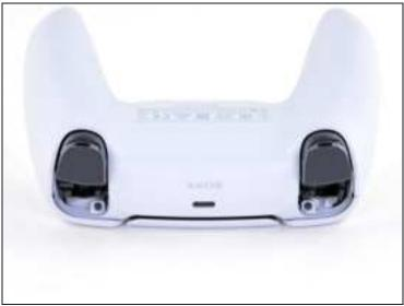
• Use a Phillips screwdriver to remove the two 6.4 mm screws behind the **L1** and **R1** buttons.
