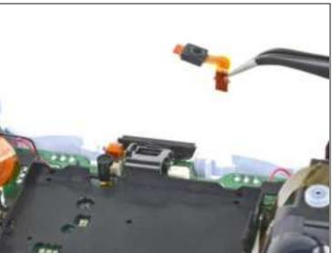
• Grab the lower microphone ribbon cable pull tab with your fingers or a pair of tweezers and disconnect it from the motherboard.
