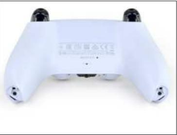
• Use a Phillips screwdriver to remove the two 6.4 mm screws securing the bottom corners of the lower case.
