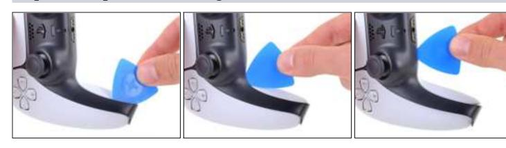
• Slide the opening pick along the lower-left edge of the middle trim to release the clips securing it to the case.
