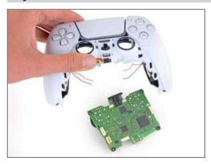
• Separate the controller from the motherboard.
