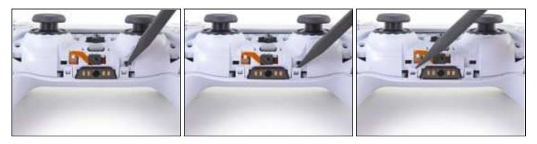
⚠ Be gentle when releasing the rear cover clips—they're delicate and can easily break.
