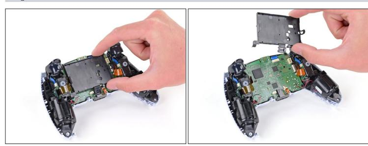
• Lift the battery bracket out of the motherboard.
