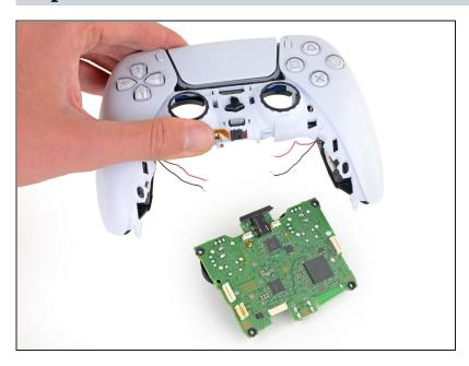
• Separate the controller from the motherboard.
