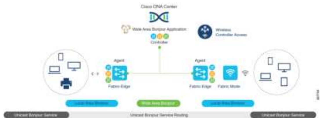
Figure 57: Cisco SD-Access Wired and Wireless Network Design
