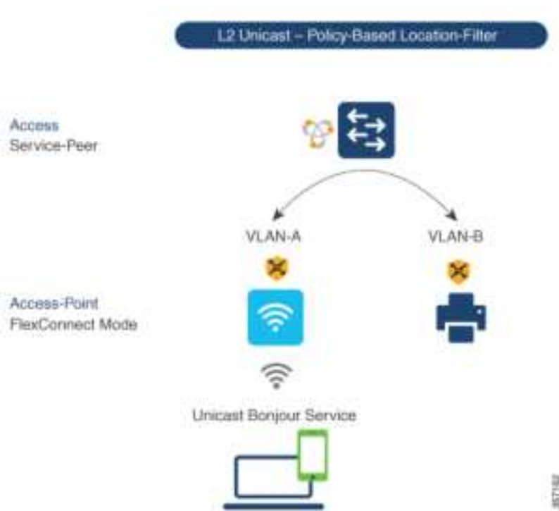
Figure 71: Catalyst Service-Peer mDNS Location-Filter Configuration
