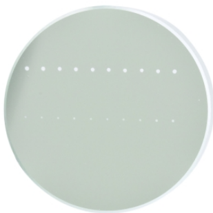
Figure 37A This photograph shows a protected aluminum-coated mirror after LIDT testing. In this particular test, it handled 0.43 \text{ J/cm}^2 (1064 nm, 10 ns pulse, 10 Hz, Ø1.000 mm) before damage.
