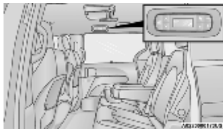
Rear Automatic Climate Controls
