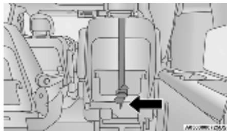
Tether Strap Anchorages (Second Row 7 Passenger Stow 'n Go Anchorage Shown)
