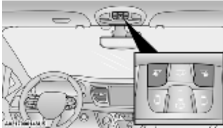
Courtesy Light Switches
