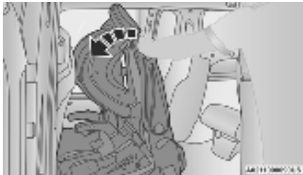
Easy Tilt With Child Seat Installed
