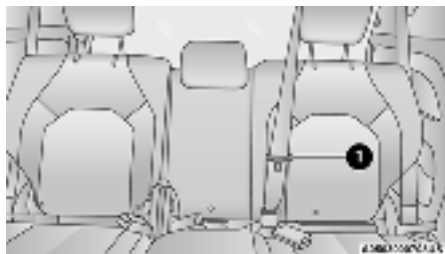
Routing The Rear Seat Belt Latch Plate
