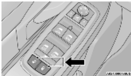
Driver Power Door Lock Switches
