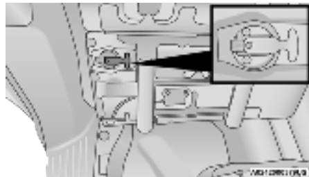
Storage Bin Cover Emergency Release Lever
