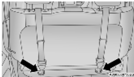
Top Tether Anchorage Locations 2nd Row Bench
