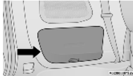
Vacuum System Access Panel
