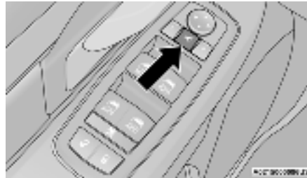
Power Folding Mirror Switch
