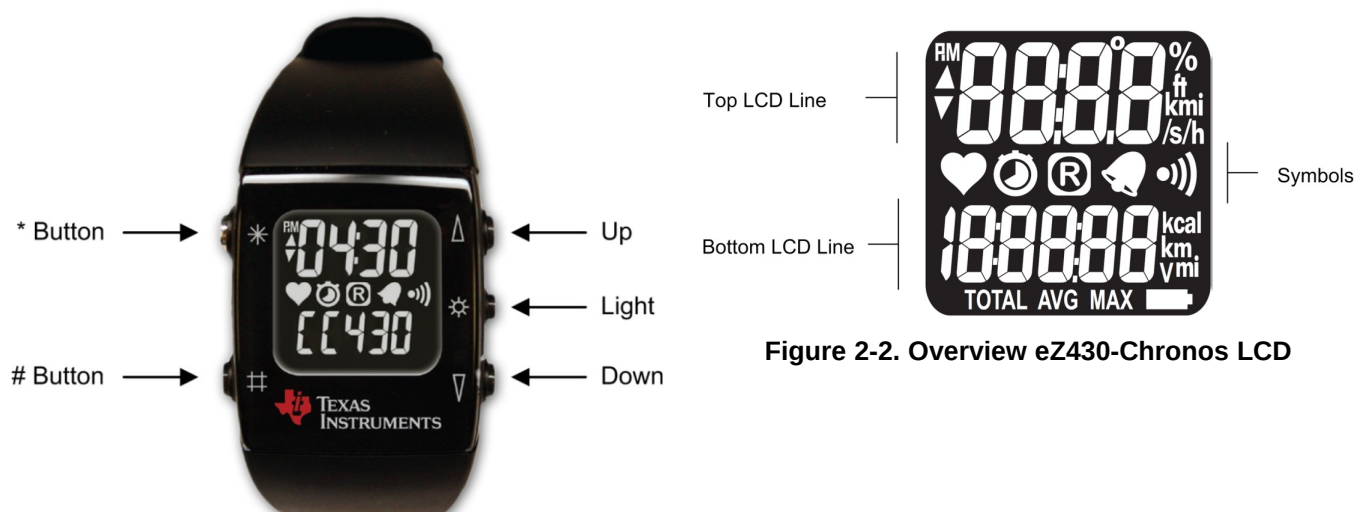
Figure 2-1. eZ430-Chronos Watch Push Buttons
