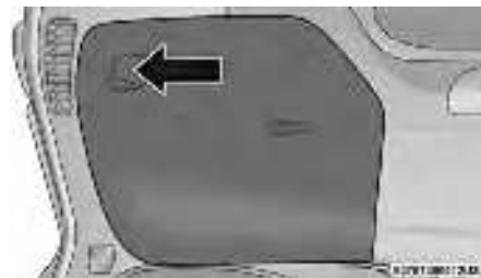
Jacking Equipment Location
