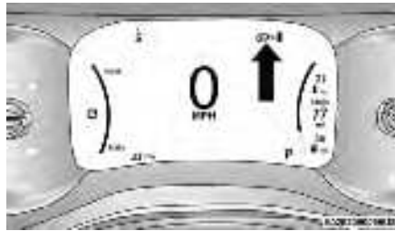
High Voltage Battery Display
