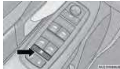
Window Lockout Switch
