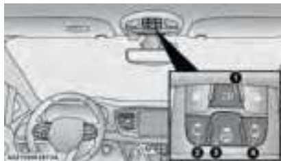
Overhead Console Power Switches
