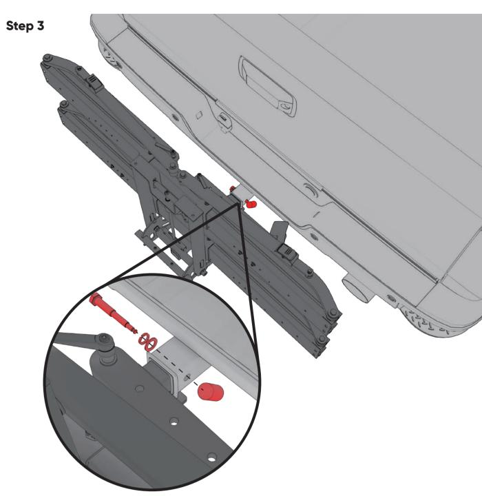
Insert the Bike Rack into the vehicle receiver and Place an **Pin Lock (4)**, through the Spring Washer and Flat Washer and the aligned holes. Insert the lock head and ensure it is securely fastened.
