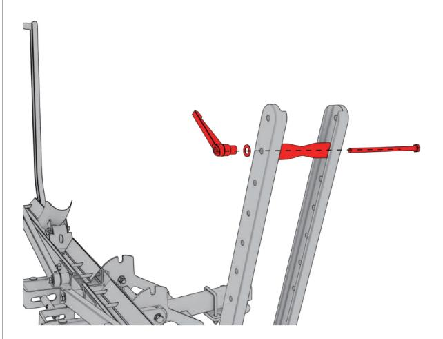
The position of the Adjustment Lever can be adjusted according to your needs. Loosen it counterclockwise and tighten it clockwise.
