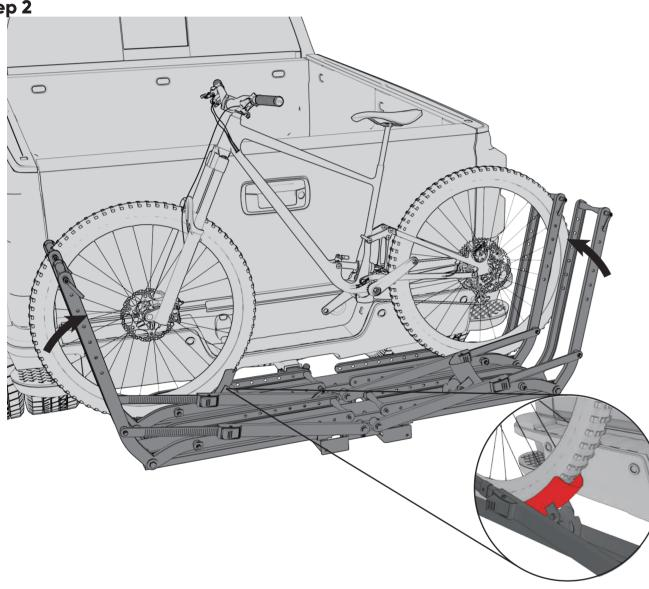
Install the bicycle on the Bike Rack, place the front wheel against the Front Wheel Holder, and tighten the Bent Arms on both sides to ensure that the front and rear wheels of the bicycle are firmly fixed.
