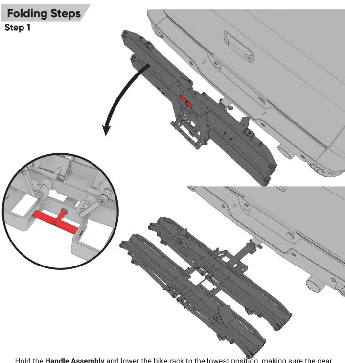
Hold the **Handle Assembly** and lower the bike rack to the lowest position, making sure the gear is correct
