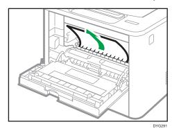
6. Slide the print cartridge in horizontally. When the cartridge can go no further, raise it slightly and push it fully in. Then push down on the cartridge until it clicks into place.
