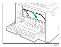
8. Slide the print cartridge in horizontally. When the cartridge can go no further, raise it slightly and push it fully in. Then push down on the cartridge until it clicks into place.
