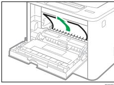
16. Slide the print cartridge in horizontally. When the cartridge can go no further, raise it slightly and push it fully in. Then push down on the cartridge until it clicks into place.
