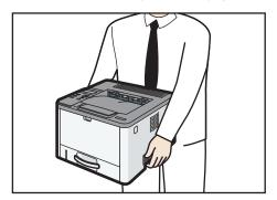
4. There are three upright pins on the optional paper feed unit. Align the holes of the machine with the pins, and then lower the machine slowly.
