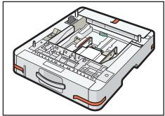
3. Lift the machine using the inset grips on both sides of the machine.
