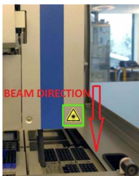
¶ Position 2 for laser light warning label (AS).
