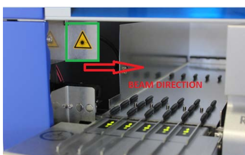
§ Position 1 for laser light warning label.
