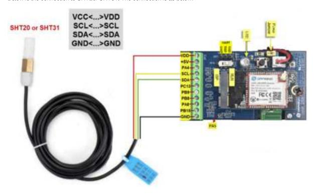
The device will be able to get the I2C sensor data now and upload to IoT Server.
