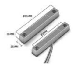
When the two pieces are close to each other, the 2 wire output will be short or open (depending on the type), while if the two pieces are away from each other, the 2 wire output will be the opposite status. So we can use SN50v3-LB interrupt interface to detect the status for the door or window.
