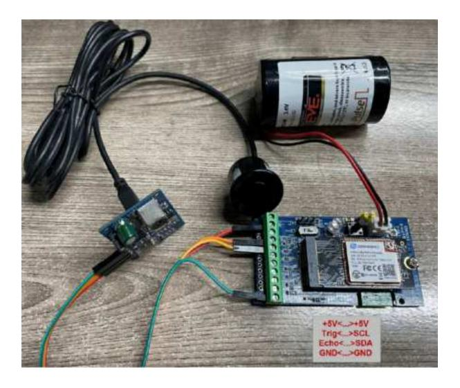
Connect to the SN50v3-LB and run AT+MOD=2 to switch to ultrasonic mode (ULT).
