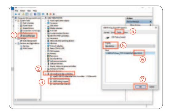
At this point, you will see that the USB port assigned to the printer by Windows is USB00\*.
