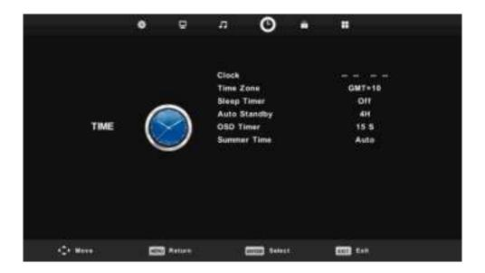
**Clock:** Display either the DTV signal stream time or set the system time.
