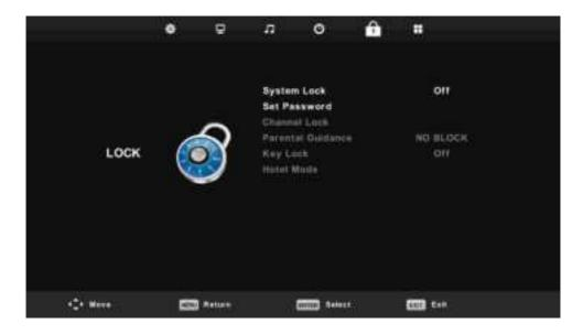
**System Lock**: The feature can prevent unauthorized operating the TV set, unless entering 4-digit password.
