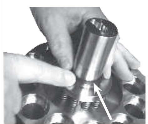
3. Assemble the O-ring over the retainer.
