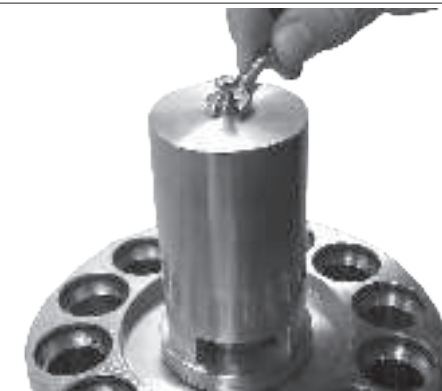
4. Using the tool provided, press down the retainer by tightening the nut until the O-ring is placed in the recess. If needed use a small screwdriver to get the O-ring into the recess.
