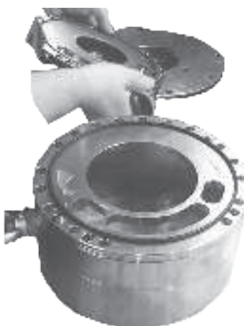
14. Remove the HP outlet flange.
