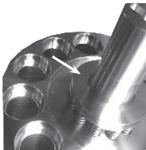
2. Assemble the retainer over the springs.
