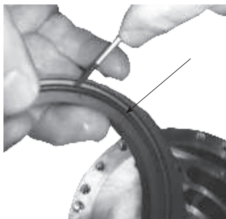
12. Remove the O-ring from the sealing plate.
