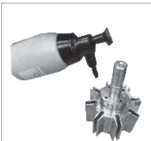
13. Place the rotor with the shaft pointing upwards and lubricate the grooves with water.
