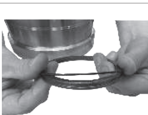
14. Install the O-ring on the rotor element.
