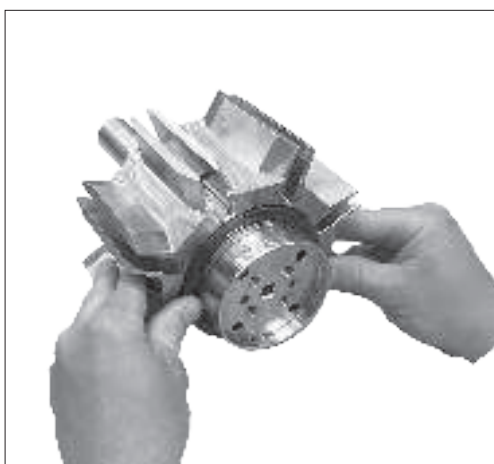
11. Carefully press the rotor element in place.
