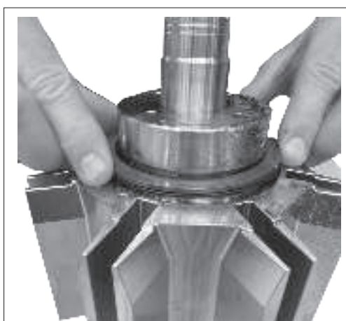
15. Place the rotor element with the O-ring installed in the groove and press down.
