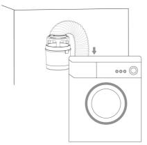
8.If your dryer is close to the wall, we recommend that you purchase a metal 90 degree elbow for yourself and install it on the dryer to avoid damage and poor exhaust due to folding of the exhaust pipe.
