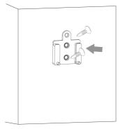
6.Insert the tank connector into the groove of the plastic clip to complete the fixing of the dryer vent.
