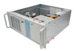
5. Lift the drive cage completely out of the device.
