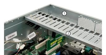
5. Loosen the bracket by unscrewing its screw ① and place it ② on the expansion card.
