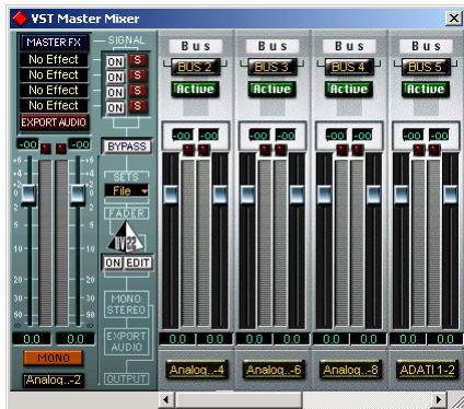
Figure 6-3: Use the output buttons at the bottom of each channel strip to assign MOTU 828 outputs to busses. You can then assign channels in the Monitor window to each bus as desired.
