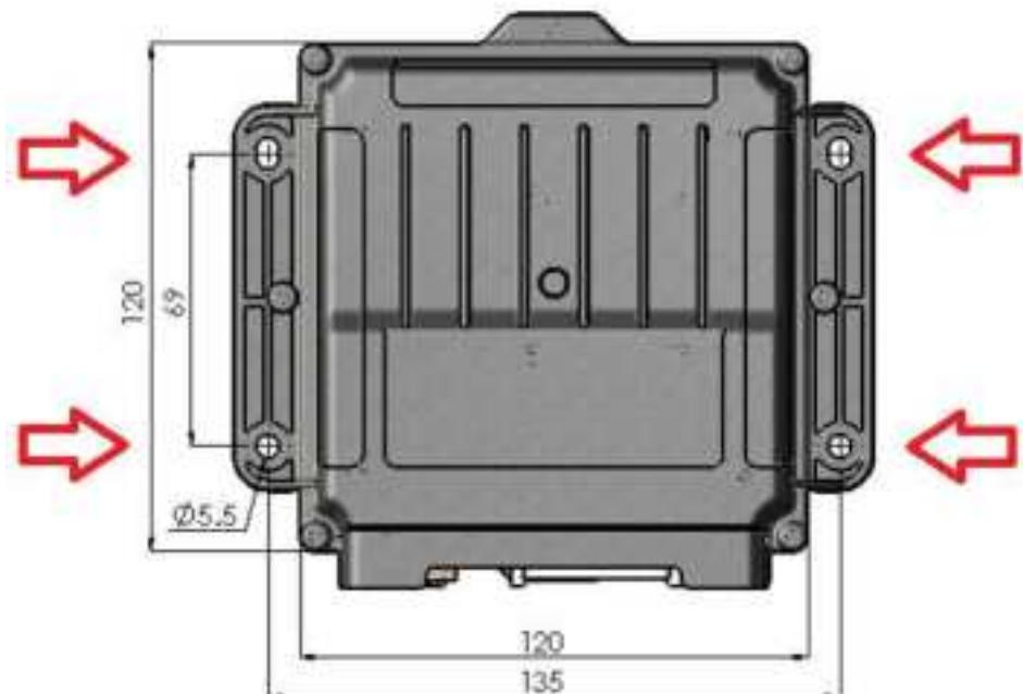
Fastening screws (M5 bolts) and washer are provided.
