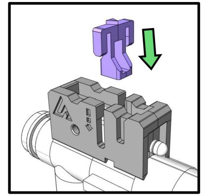
**D10.** Once installed try using a rod to move the trolley up and down and ensure it can do so easily without much resistance.
