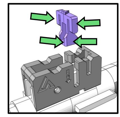
**D9.** Orientate the trolley to face the front, you can use the arrow located at the top to find the orientation and insert into the TDC Bracket.
