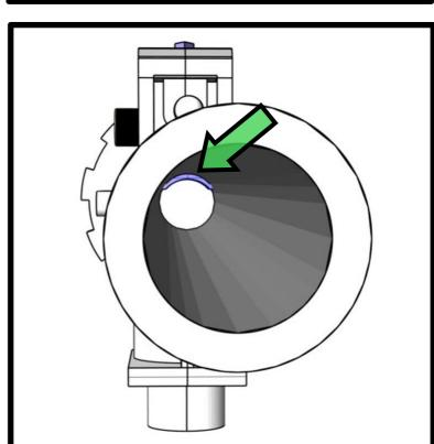
**D18.** If youre happy with the set up and everything is working, you can superglue/ Loctite the bracket set onto your hop up chamber. Only the lower edges is required. But please don't glue until you are fully happy with the set up!
