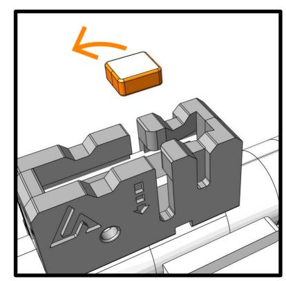
**D**7. Place the M-nub into the hop-up window inside the chamber
