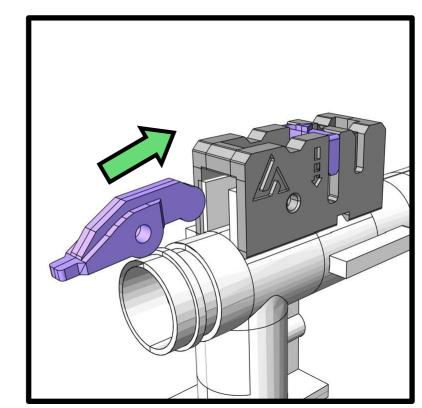
**D12.** The adjustment arm will be installed the middle of the TDC trolley as shown in the diagram.
