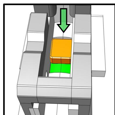
**D8.** Apply silicone grease on all the surfaces that will come in contact with each other or the TDC operation. All vertical surfaces should be applied.
