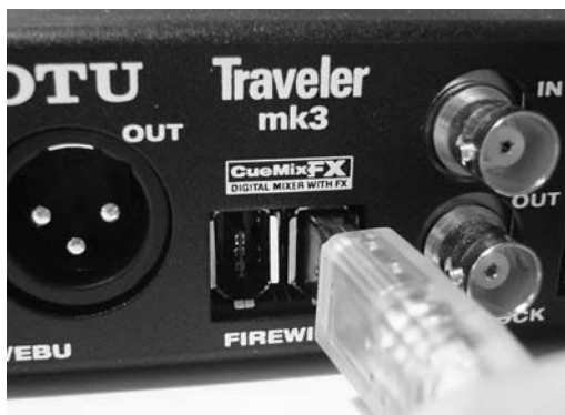
Figure 3-1: Connecting the Traveler-mk3 to the computer.
