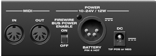
Figure 3-10: The Traveler-mk3's battery and power supply options.
