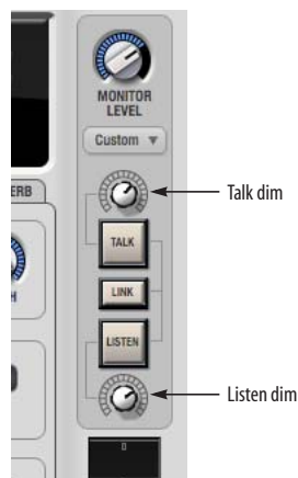
Figure 11-31: The Talkback/Listenback controls.
