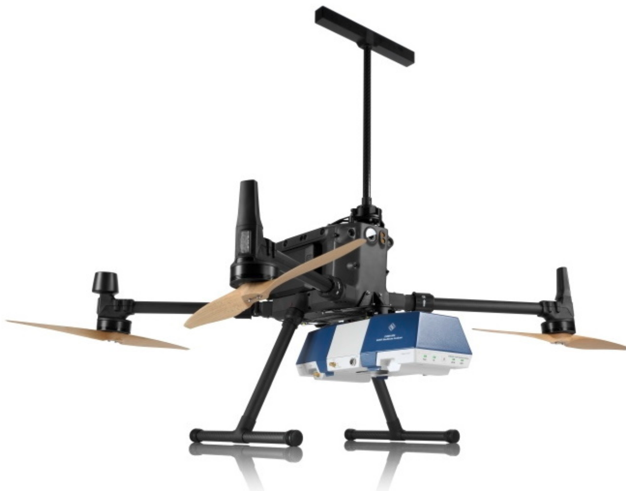
Figure 4-1: Example of a R&S EVSD1000 mounted to a DJI M300 drone
