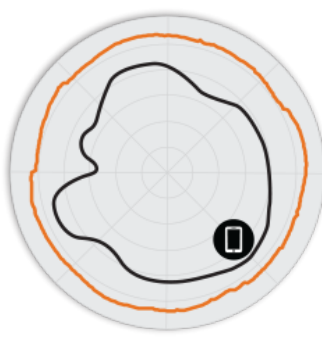
Figure 3. R730 5GHz AzimuthAntenna Patterns
