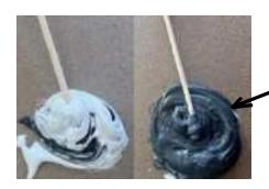
3rd mix the 2-part epoxy until you get the desired color instructed with this epoxy mix that it's been fully mixed, and ready to use.
