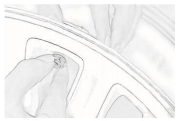
Step 2: Fix the sensor on the air nozzles with the sensor fixing screw. Note that the sensor should be close to the hub with a torque of  $4N \cdot m$ .
