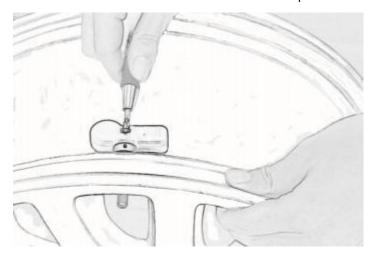
Step 3: Tighten the air nozzle fixing nut with a wrench to complete the installation. Note that the wrench uses a torque of 7  $N \cdot m$ .
